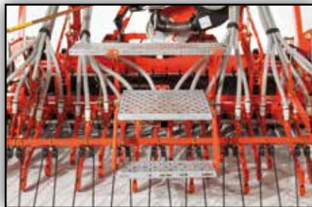
Loading step for safe and secure hopper filling
