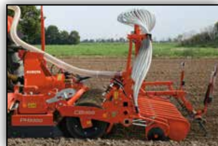
The coulter bar is attached to the harrow via the coulter toolbar linkage. This ensures to maintain a constant seeding depth. The rapid coupling system allows the power harrow to be converted easily for solo use.
