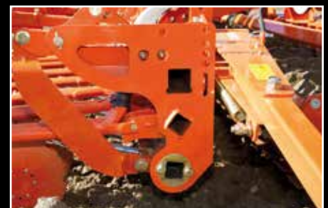
Overload protection of the marker arm
