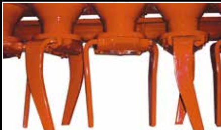
Fully welded rotor housings ensure high bending and torque resistance to the trough when working in very tough soil conditions. This also provides an optimum clearance between the trough bottom and tine holders and allows large amounts of residues and stones to pass freely without blocking.
