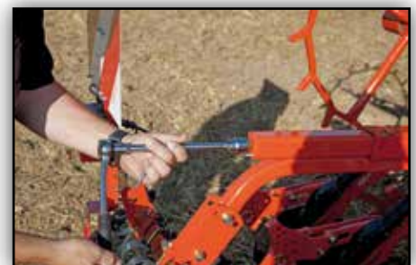
Depending on the soil conditions the pressure and angle of the following harrows can be adjusted manually.
