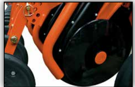
CX-II coulters with double entry for fertiliser application (red tube) and seeding (black tube) in one pass.
