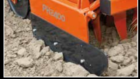
Floating side deflectors with overload protection allow smooth operation and a ridge free soil surface.
