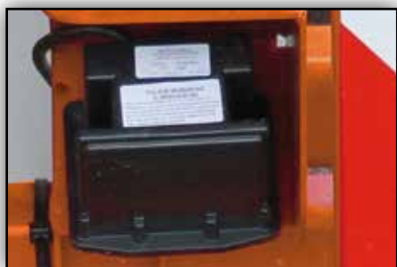
An optional available radar speed sensor can simultaneously record the speed SH1150 in order to maintain the relevant distribution rate at the correct time.
