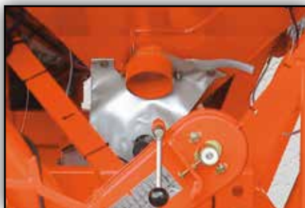
A large emptying chute directly above the metering device allows quick removal.
